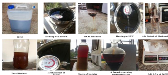
Figure 3: Process of biodiesel production.
