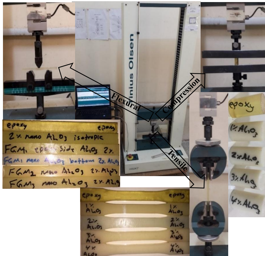
Figure 4: Universal testing machine and samples used
