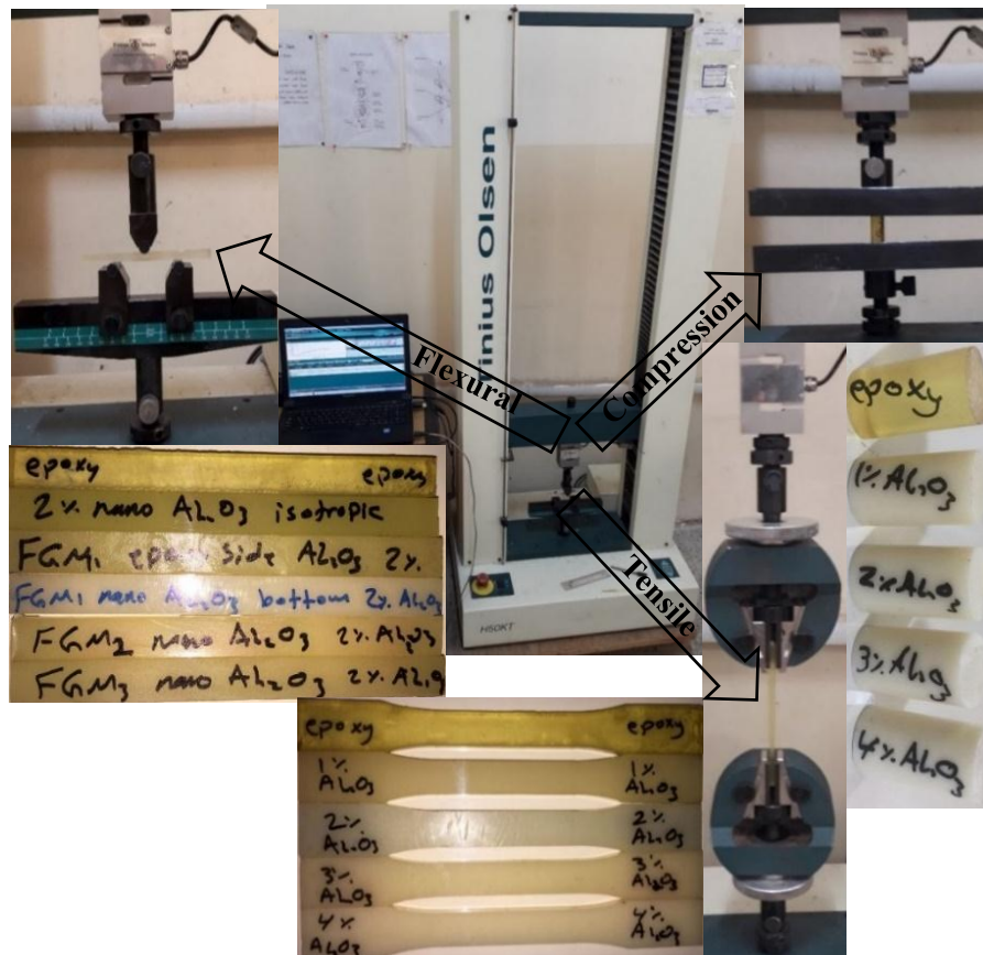
Figure 4: Universal testing machine and samples used
