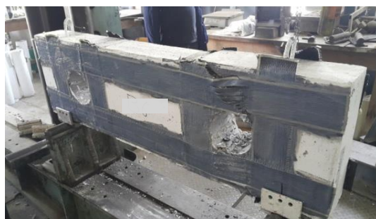
Plate 5: Failure mode and tearing of CFRP strip for B3-R-VH
