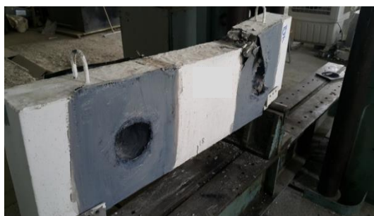
Plate 7: Failure mode and tearing of CFRP strip for B5-R-SS
