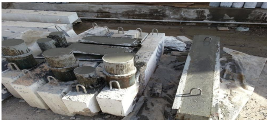
Plate 1: Deep beam specimens and control specimens after finished casting process
