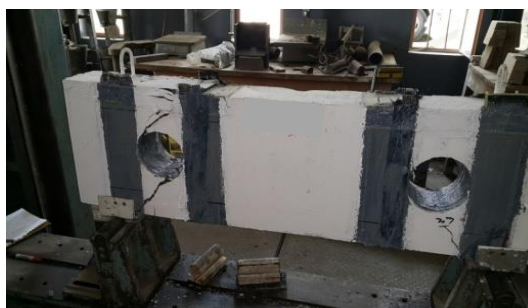
Plate 3: Failure mode and cracks patterns for B1-R-V
