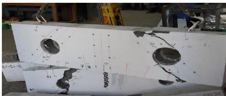
Plate 2: Failure mode and cracks patterns for B1-Control
