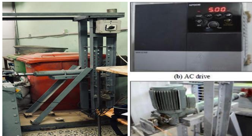
Figure 5: Horizontal movement device used in the test.
