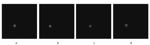
Figure 3: The gray scale of the spot of the output light with different concentration surrounded the PCF. (a) Output light with distal water. (b) spot image at 1% zinc concentration. (c) spot image at 2% zinc concentration. (d) spot image at 3% zinc concentration
