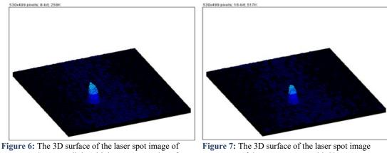
igure 6: The 3D surface of the laser spot image of the output light with low concentration of 1% Zn surrounded the PCF
