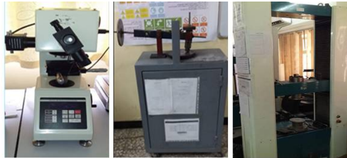
Figure 1: Digital Micro Hardness Tester, Dry sliding wear machine, Compressive test machine
