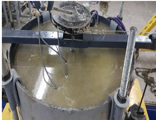
Plate 4: liquefaction phenomena occurred after applying 0.32g acceleration
