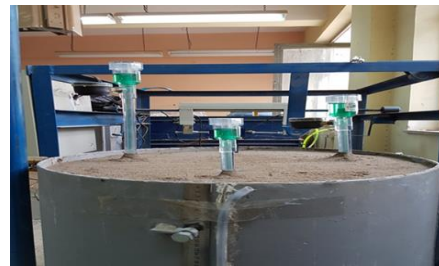
Plate 2: Soil suction test by LT Tensiometer
