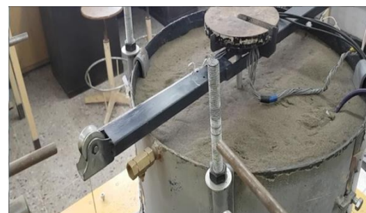
Plate 3: Single pile embedded in unsaturated soil subjected to lateral shaking load (earthquake). Single phenomena occurred after applying 0.32g acceleration
