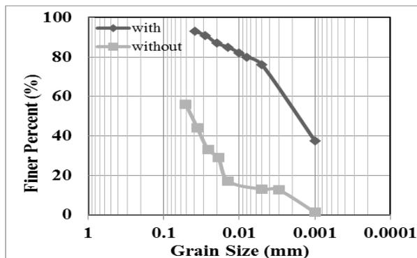
Figure 2: Grain size distribution for dispersive clay with 5% Na<sub>2</sub>CO<sub>3</sub>
