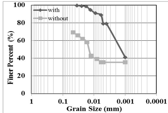
Figure 5: Grain size distribution for dispersive clay with 30% Na<sub>2</sub>CO<sub>3</sub>
