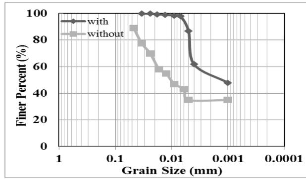
Figure 4: Grain size distribution for dispersive clay With 25% Na<sub>2</sub>CO<sub>3</sub>
