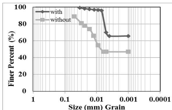
Figure 7: Grain size distribution for dispersive clay with 40% Na<sub>2</sub>CO<sub>3</sub>
