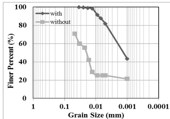
Figure 3: Grain size distribution for dispersive clay with 15% Na<sub>2</sub>CO<sub>3</sub>
