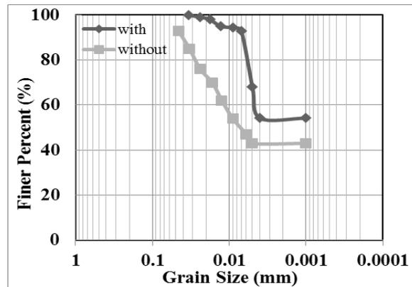
Figure 6: Grain size distribution for dispersive clay with 35% Na<sub>2</sub>CO<sub>3</sub>
