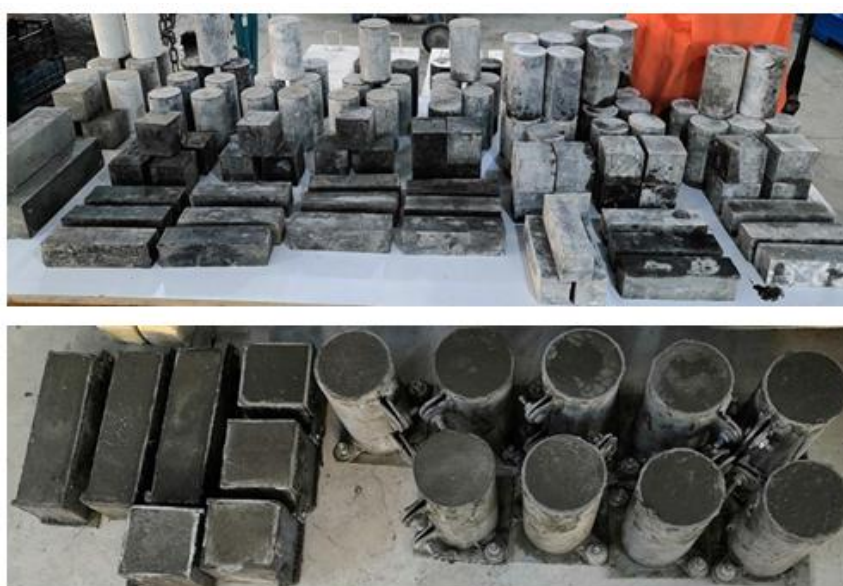
Figure 4: The UHPC specimens that were prepared for testing
