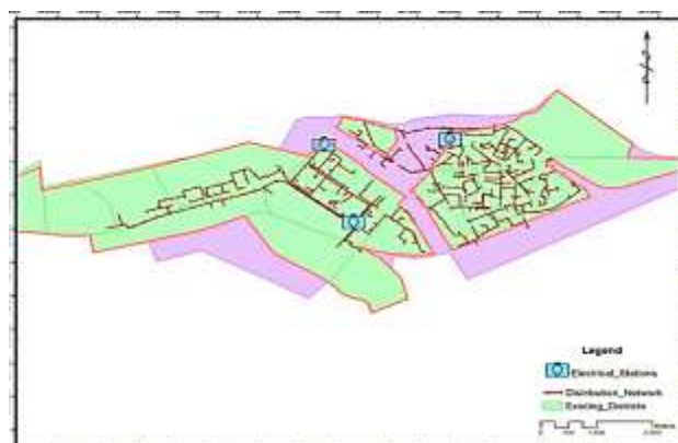
Figure 3: Map of Existing Electrical Distribution Network
