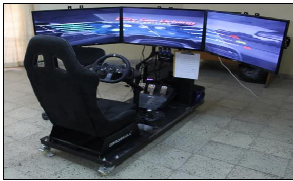
Figure 2: Driving simulator device
