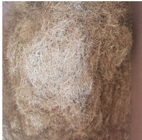
Plate (1): Micro Steel Fiber
