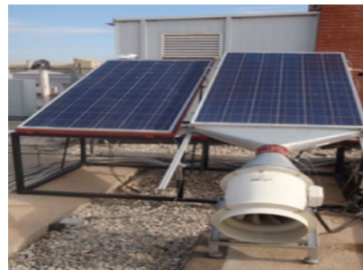
Figure 7: PV cooling by forced air.
