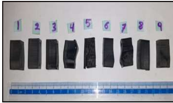
Figure 4: Deformation in samples of each run after being subjected to compression test
