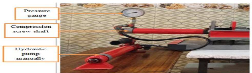
Figure 3: Parts of the compression system
