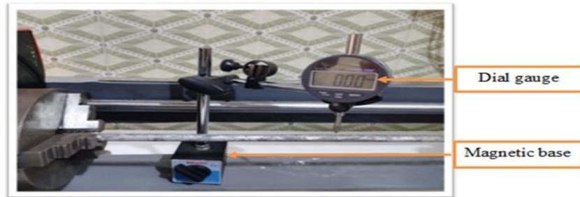
Figure 5: Buckling failure measuring device
