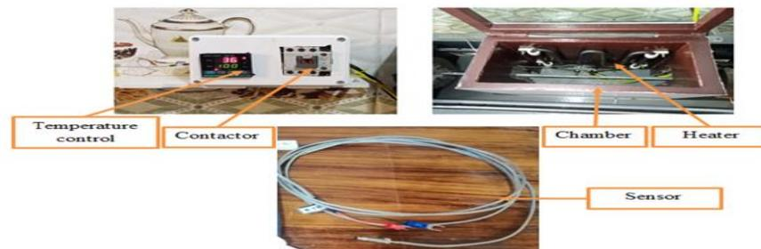
Figure 4: Parts of the electric oven
