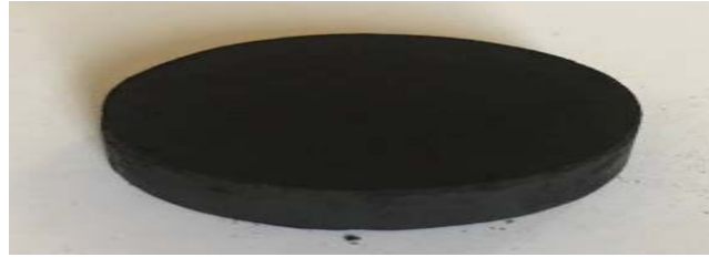
Figure 1: The pellet of \text{Fe}_3\text{O}_4 20 mm diameter and thickness of 6 mm
