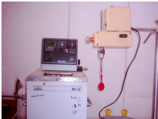
Figure 2: Electric mixer with four blades, plastic impeller
