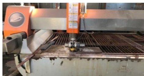
Figure 1: Experimental setup for abrasive water jet machining
