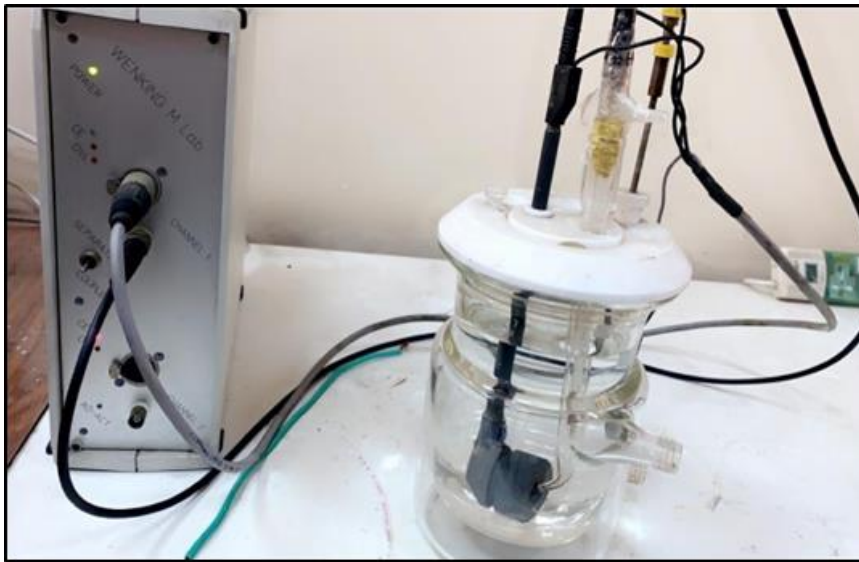
Figure 2: Figure 2: The cyclic potential dynamic polarization test device
