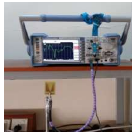
Figure 8: Return loss measurement of the antenna using ZVA 13 vector network analyzer.
