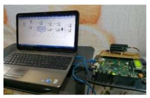
Figure 9: Hardware connection Spartan-3A DSP 3400A and hosting computer
