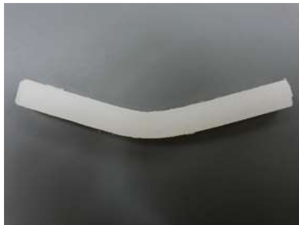
Figure 25: Specimen after bending test
