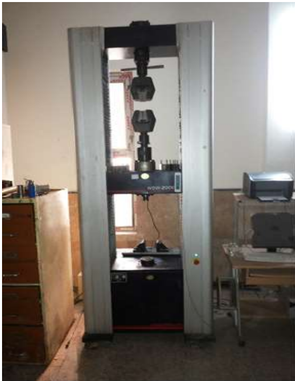
Figure 15: Tensile test machine type (WDW-200E)
