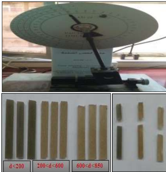
Figure 5: Impact device and samples of specimens before and after test.
