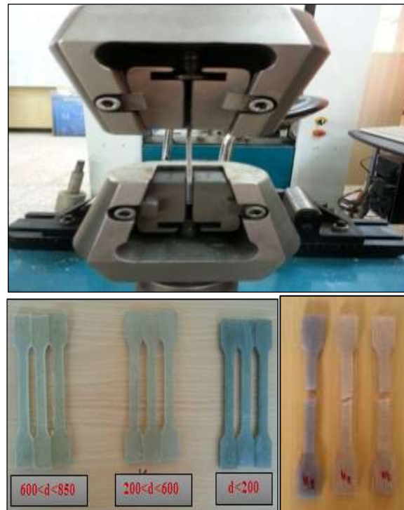
Figure 3: Tensile device and samples specimens before and after test.
