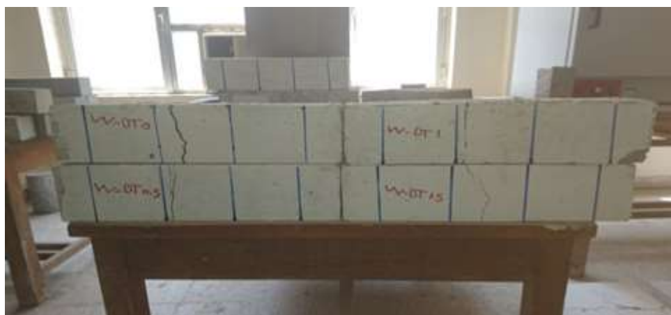
Figure 7: Modes of failure of concrete prisms
