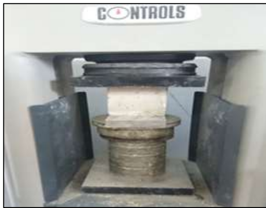
Figure 4: Compressive Strength test
