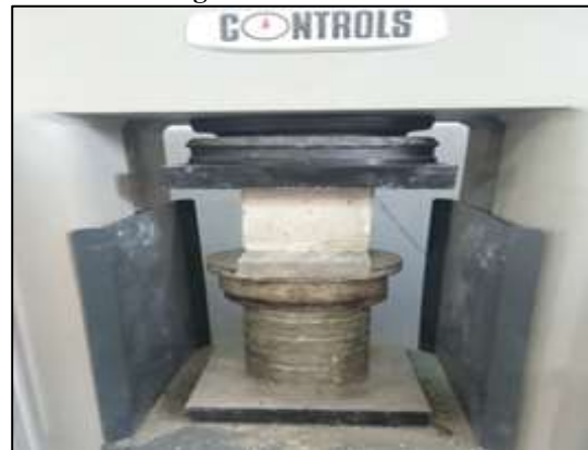
Figure 3: Splitting Tensile test
