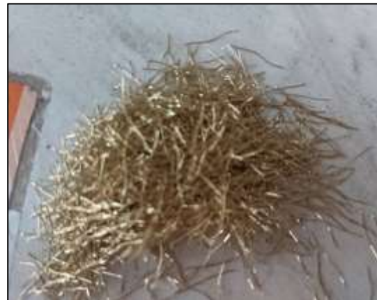
Figure 1: Steel fiber used in constructing the specimens.
