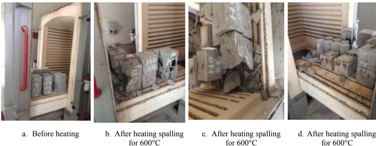
Figure 11: Samples before and after heating in the electric oven
