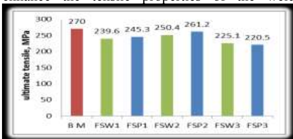
Figure 8: Tensile test results
