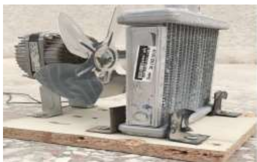
Figure 5: Fan and cooling coil unit
