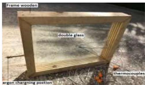
Figure 4: Test section frame of glasses
