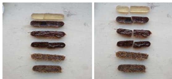
Figure 3: Impact test experimental specimens 1-pure Epoxy, 2-Epoxy+5%CS, 3-Epoxy +10%CS, 4-Epoxy +15%CS, 5-Epoxy +20%CS, 6-Epoxy+25%CS
