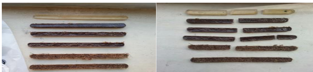
Figure 4: Flexural Strength experimental specimens before & after test 1-pure Epoxy, 2-Epoxy +5%CS, 3- Epoxy +10%CS 4- Epoxy +15%CS, 5- Epoxy +20%CS, 6- Epoxy +25%CS
