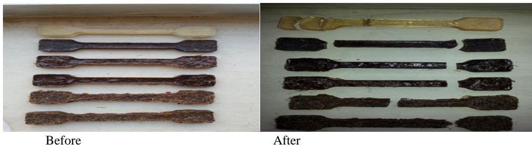
Figure 2: Tensile test Experimental specimens. 1-pure Epoxy, 2-Epoxy +5%CS, 3- Epoxy +10%CS 4- Epoxy +15%CS, 5- Epoxy +20%CS, 6- Epoxy +25%CS
