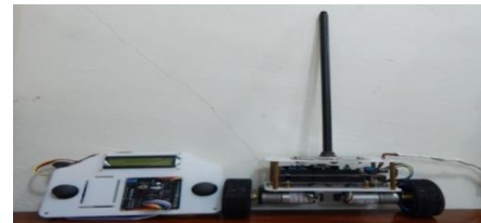
Figure 3: The constructed real two wheeled inverted pendulum system.
