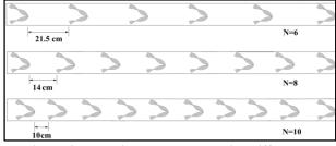
Figure 3: Inserting turbulators with different values of N
