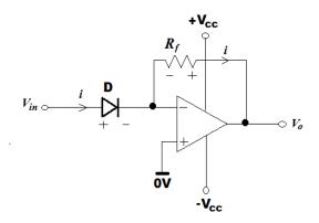
Figure 2: Circuit diagram of the anti-logarithmic amplifier
