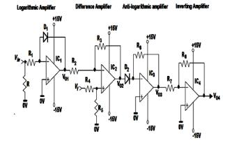
Figure 3: Circuit diagram of the proposed system
