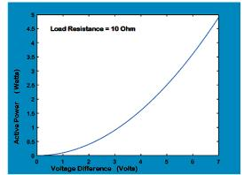
Figure 8: The result of relation between the actual power and the applied voltage of the work of Ilsche *et al.* [9]
