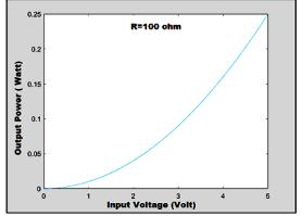
Figure 7: The result of relation between the actual power and the applied voltage of the work of Mahmud *et al.* [8]
