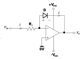
Figure1: Circuit diagram of the logarithmic amplifier
