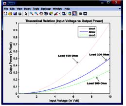
Figure 5: Theoretical relation between consumed power and applied voltage using the proposed circuit
