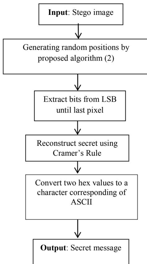
**Figure2: Block diagram for extracting text file of proposed method**
