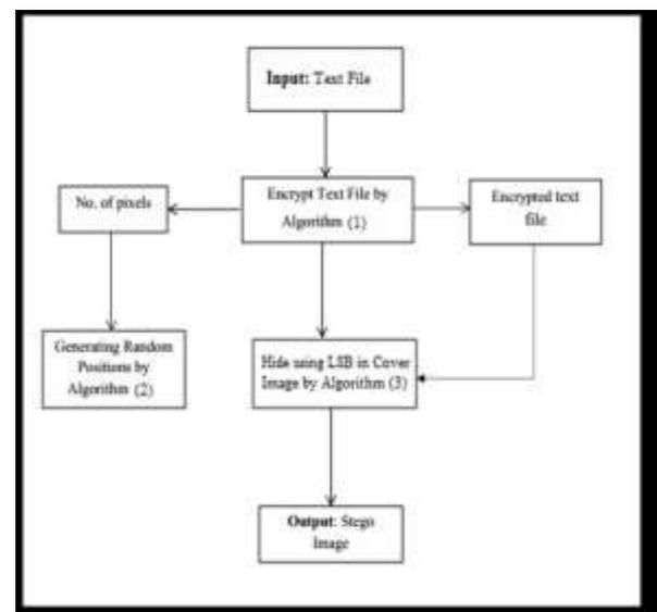
Figure 1: Block diagram for text file hiding method
