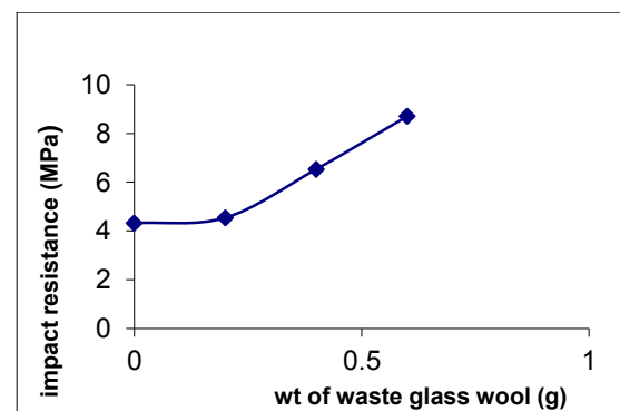
Figure 3: Impact Resistance as a function of wt. of waste wool glass (g)
