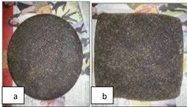
Figure 1: Shows a: the base polyester, b: polyester reinforced waste glass wool specimen.
