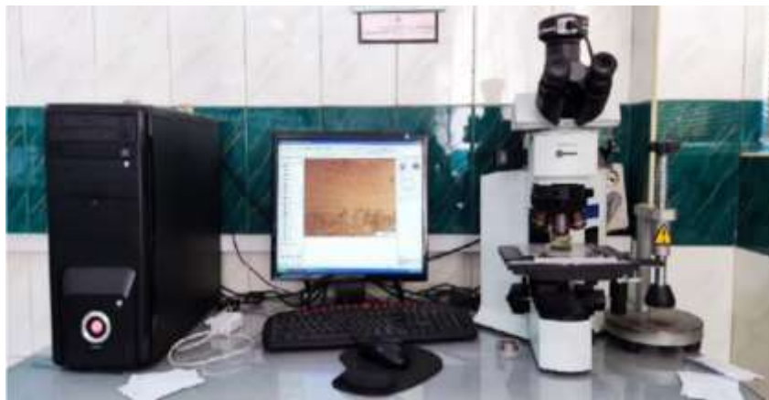
Figure 6: Optical Microscope (Olympus BXM51) equipped with digital camera and image processing software
