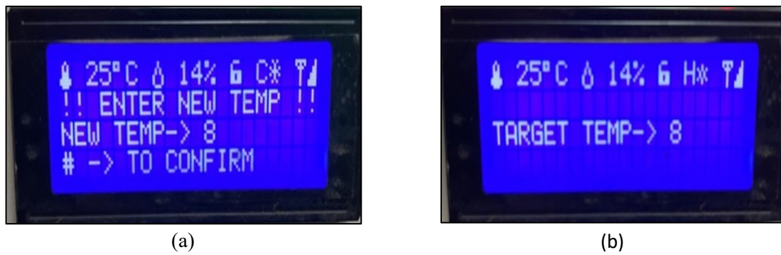
Figure 5: The settings function and automation preservation of the target temperature. (a) using the letter C, (b) show target temperature
