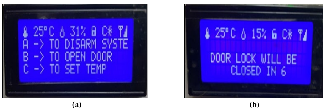
Figure 4: Opening of the cube door. (a) use of letter B, (b) the door is opening
