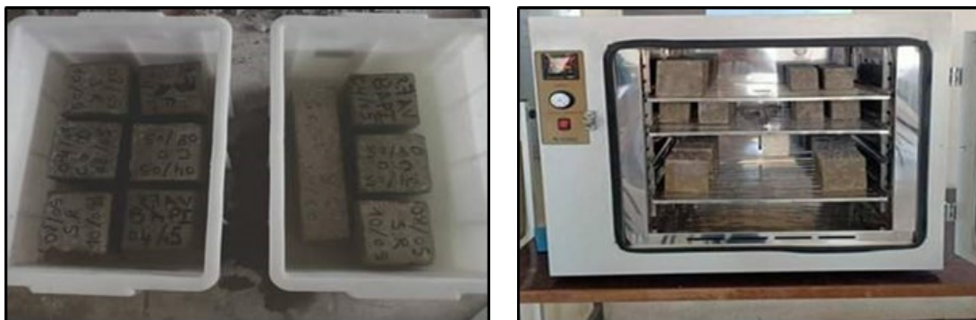
Figure 6: Samples placed in the saline solution: a) Immersion of the specimens b) Drying in the oven at 60^\circ
