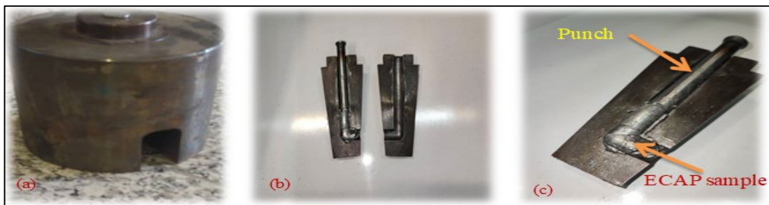
Figure 7: (a)Appearances of ECAP Die (b) two pieces split die parts (c)ECAPed sample during the process
