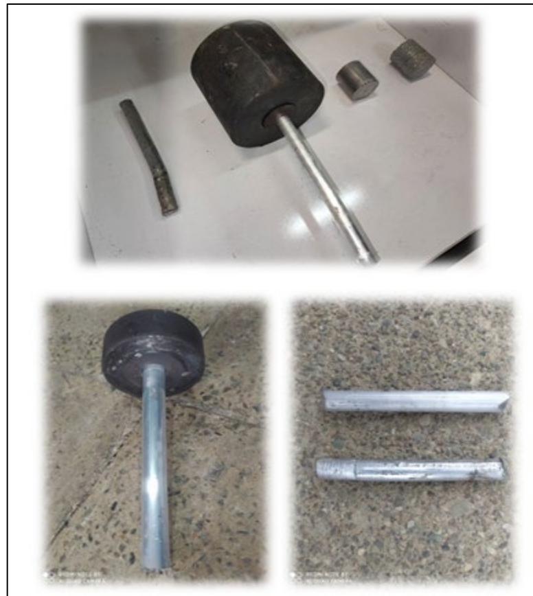
Figure 4: (15) mm diameter extruded samples of Al-6061 aluminum alloy chips
