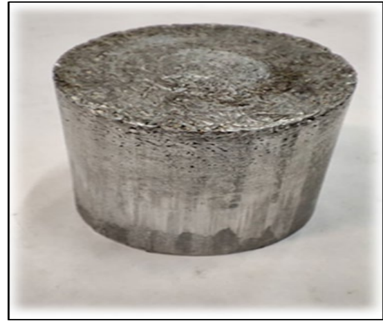
Figure 3: A compacted sample of 6061 aluminum alloy chips
