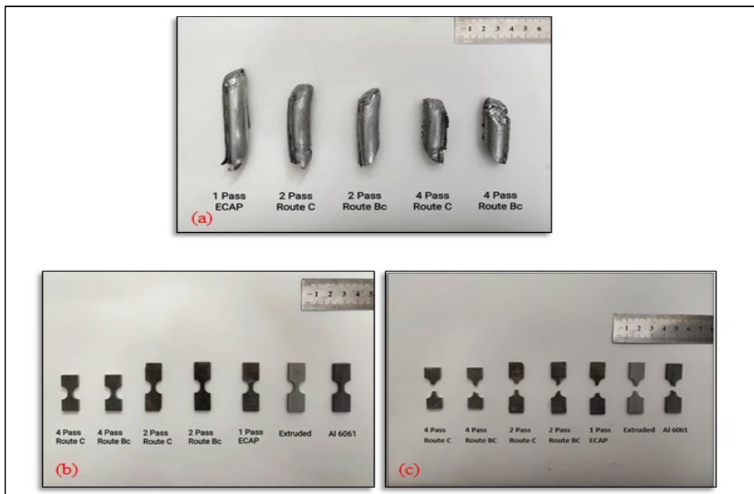
Figure 13: Actual specimens' appearance; (a) Various samples following ECAP preparation and (b) Tensile test samples; and (c) After a tensile test, the specimens were fractured
