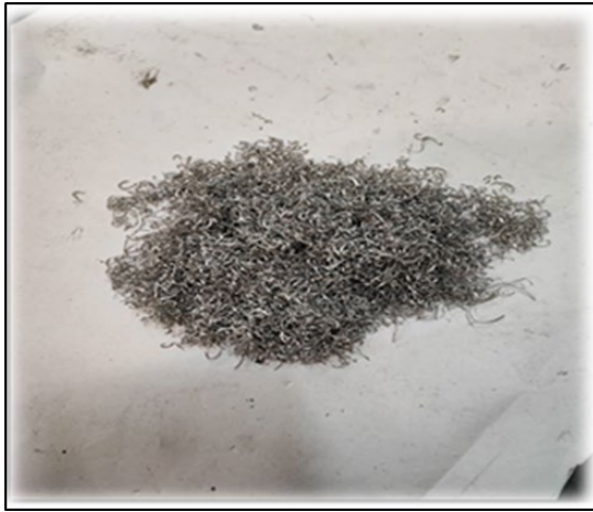
Figure 2: Al-6061 alloy prepared of chips
