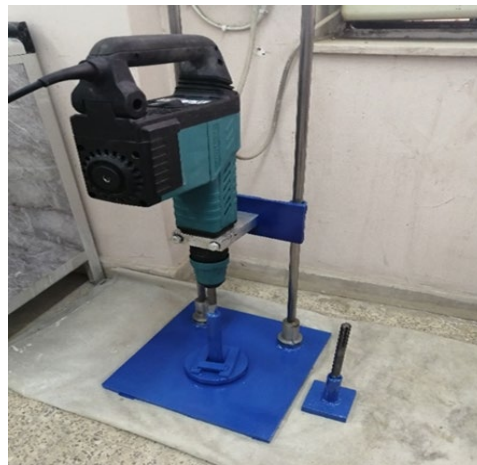
Figure 1: Vibration hammer for RCC sampling
