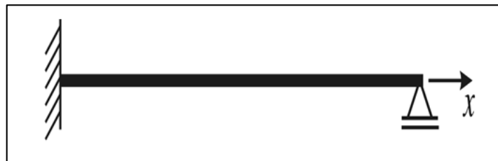
Figure 4: Thin beam with clamped-simply supported ends
