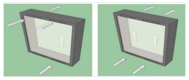
Figure 4: Illustration of the ventilation concepts: Cooling mode (left) and Heating mode (right) [38]
