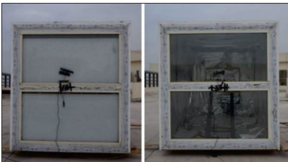
Figure 3: Experimental Setup (A) Façade Filled with PCM (B) Façade Filled with Air [22]
