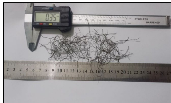
Plate 2: Steel Fibre Geometry and Shape after Recycling
