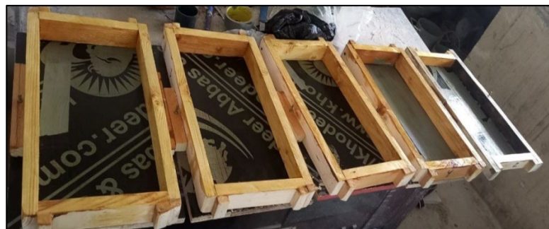
Plate 4: Wooden Molds used to Produce Geopolymer Concrete Paving Flags
