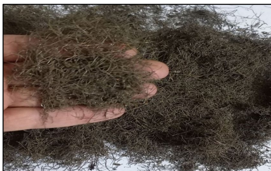
Plate 1: Recycled Steel Fibre Used in this Investigation
