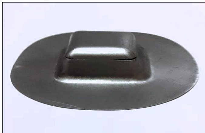
Figure 7: The failed cups from the conventional deep drawing lubricated conditions
