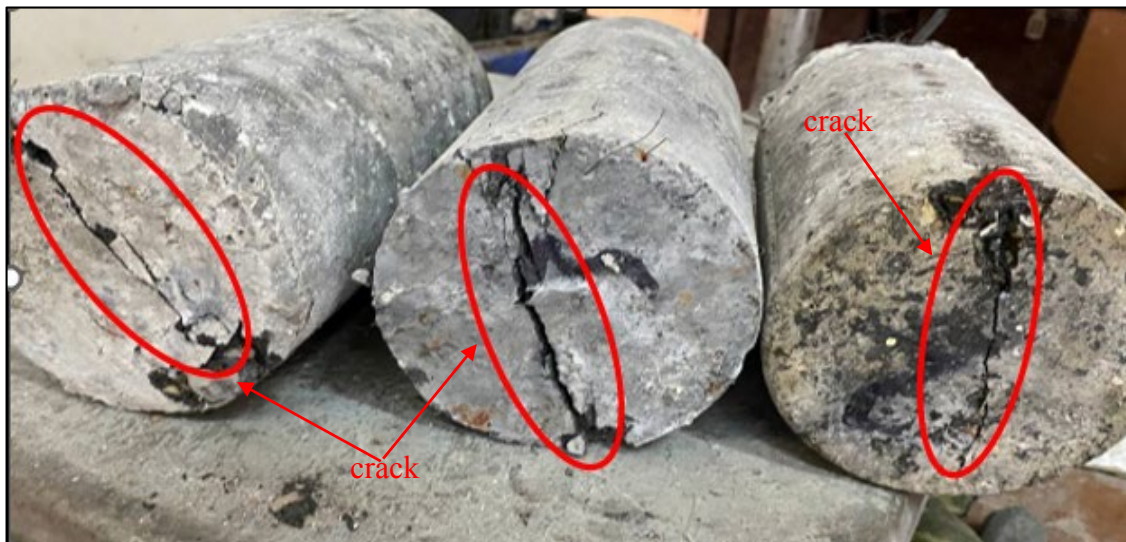
Figure 7: Failure Mode for specimen's concrete under splitting tension
