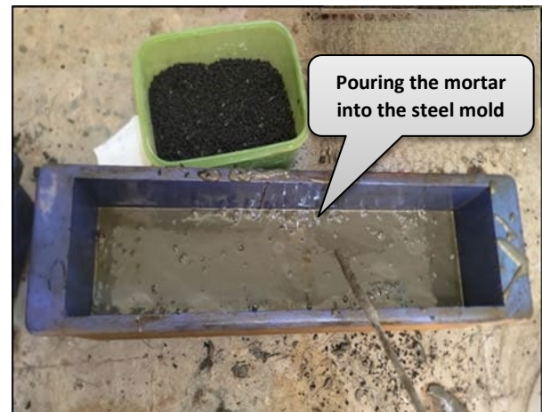
Figure 2: Casting processes of SIFCON specimens
