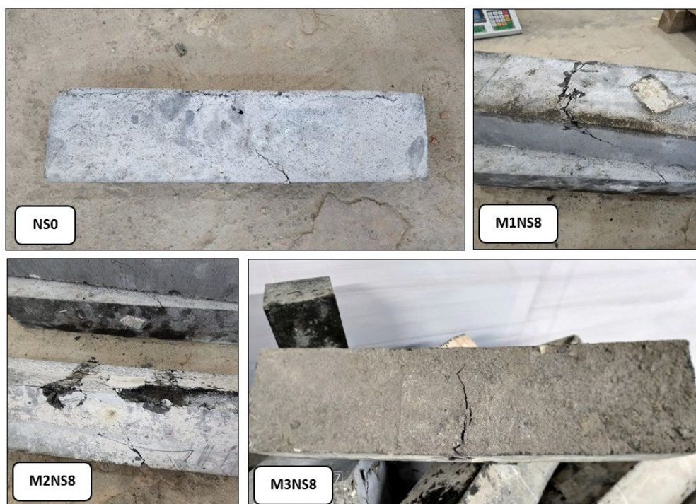
Figure 7: The flexural failure mode of SIFCON samples.
