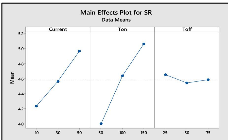
Figure 8: Main effects plot of SR using composite electrode (Cu-1%Cr-0.5%WC-1%Ag)
