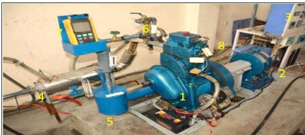
Figure 9: Front view of the experimental set up 1-Diesel engine rig test 2- Eddy current dynamometer 3- Control panel 4- Calorimeter 5- Outer surge tank 6- EGR flow meter 7- Temperature recorder 8- Magnetics setup
