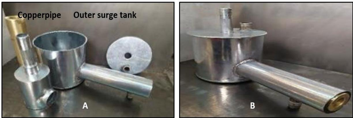
Figure 8: A- Diesel engine EGR parts and B-Diesel engine EGR parts after collection
