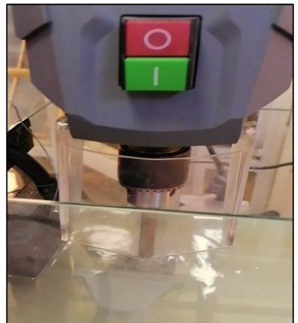
Figure 3: The workpiece is immersed in the solution tank, copper electrode, and aluminum workpiece holder
