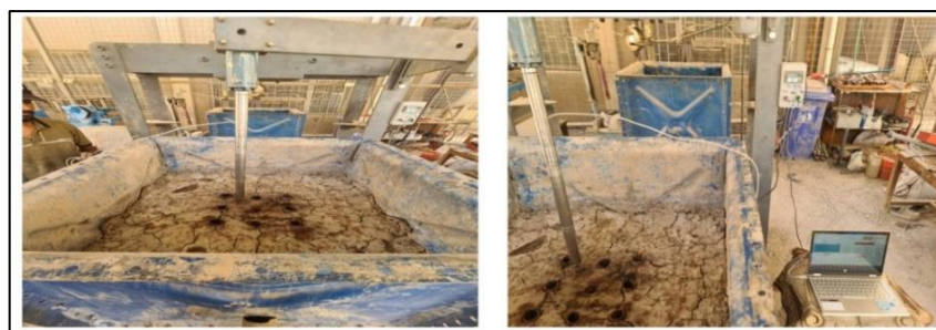
Plate 5: Prepare the CPT probe to model the test
