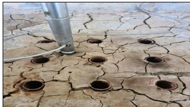
Plate 7: The end test of CPT probe depth
